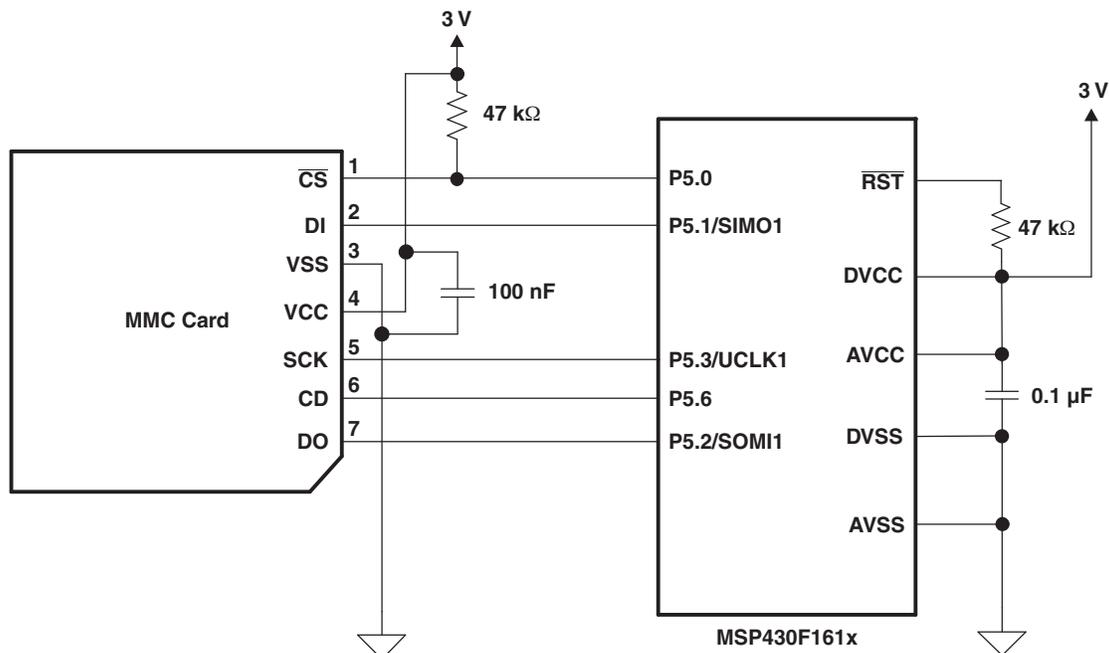
**Figure 1. Connection Between MSP430 and MMC Card**
