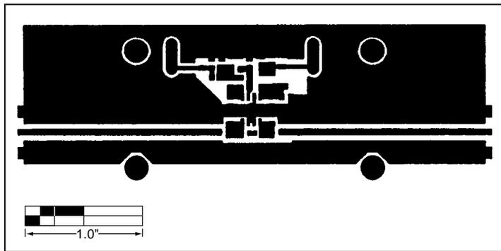
Figure 4. MAX2602 EV Kit PC Board Layout—Component Side
