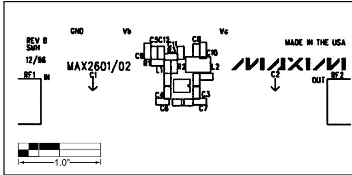
Figure 3. MAX2602 EV Kit Component Placement Guide
