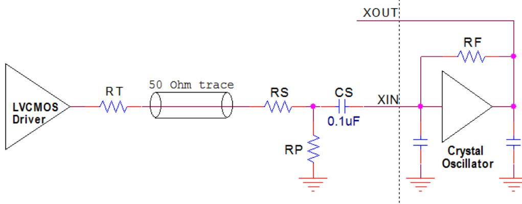
On-chip crystal oscillators are commonly designed around an inverting amplifier. There are capacitors to match the load capacitance of the crystal and a feedback resistor  $R_F$  for DC bias (see [Figure 1](#)). Instead of connecting a crystal between the XIN and XOUT pins, XIN can also be driven with a single ended clock signal. In that case XOUT will be left open. When using CS for AC coupling, the crystal oscillator's DC bias remains functional.
