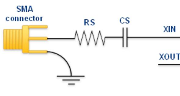
Also see “Appendix A” for optional signal adjustments for optimum performance. When the evaluation board output is AC coupled, CS will not be needed. Connect the SMA connector ground as close as possible to the IC ground pin for the crystal oscillator to avoid adding in ground noise.
